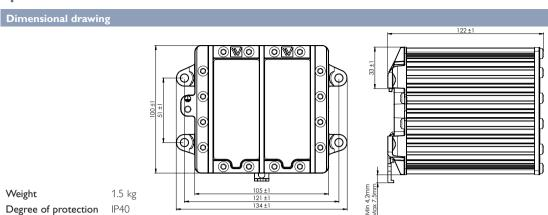
**Dimension**  $134 \times 100 \times 122 \text{ mm } (5.25 \times 3.93 \times 4.80 \text{ in})$
