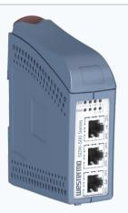
The SDW-541 is an unmanaged 5 port (4TX and 1FX) industrial Ethernet switch designed for easy use in heavy duty industrial applications. The unit supports 802.1Q long packets which allows all standard industrial Ethernet protocols to be used. A number of standard fibre optic connection types are supported including LC, SC and ST.
