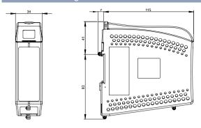
**Dimension W x H x D**  $34 \times 123 \times 121 \text{ mm} (1.33 \times 4.84 \times 4.76 \text{ in})$
