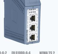
The SDW-550-T5G is an unmanaged 5 port switch with five copper ports, all supporting 10 Mbit/s, 100 Mbit/s or Gbit Ethernet. It is designed for easy use in heavy duty industrial, maritime and rail trackside applications. The unit supports 802.1Q long packets which allow all standard industrial Ethernet protocols to be used.
