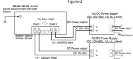
**Notes:**The recommended working voltage is DC12V/24V/48V (DC10~60V, 0.8A).
